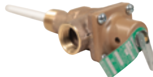
Temp & Pressure Relief Valve 210°F / 150PSI 3/4"M x 3/4"F NPT
